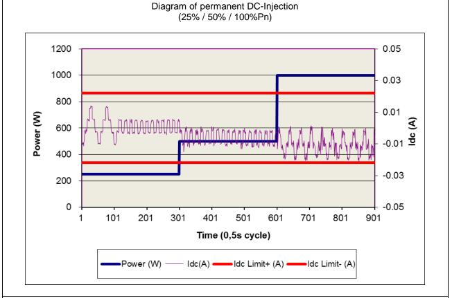
The average d.c. current injected by the embedded generator shall not exceed 0,5 % of the rated a.c. output current over any 1-minute period, into the utility a.c. interface under any operating condition.
