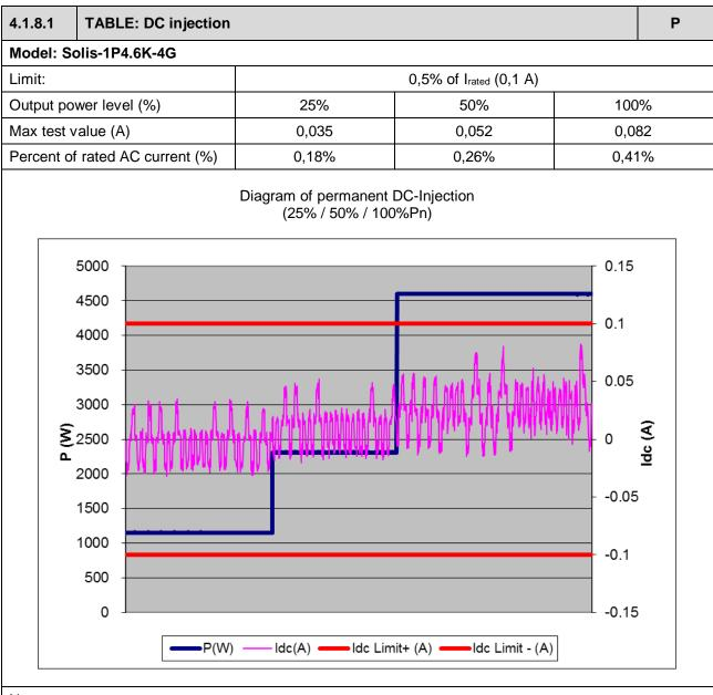
The average d.c. current injected by the embedded generator shall not exceed 0,5 % of the rated a.c. output current over any 1-minute period, into the utility a.c. interface under any operating condition.
